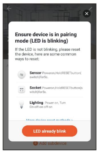
• Remove the insulation sheet and press the reset button for 5 seconds, till the blue LED blink, then click "LED already blink" on the app.
