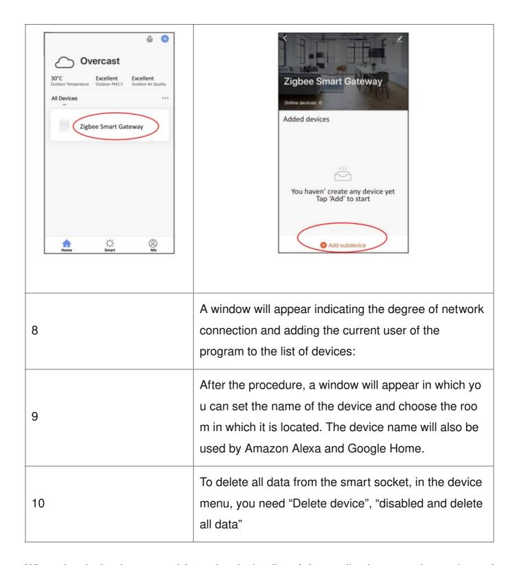
When the device is removed from the device list of the application user, the settings of the smart socket will be reset to factory values and it will be necessary to shorten the procedure of connecting to the Wi-Fi network again. If the password for the Wi-Fi access point was entered incorrectly, then after the timer expires, a "failed to connect to Wi-Fi" window appears in the application with step-by-step instructions to fix the problem.
