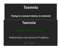
When the connection is complete, the inscription "Successfully connected to Wi-Fi" and the address of your device on the network will appear
