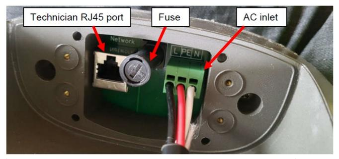
• Close back compartment cover, tighten 4 captive screws and then tighten cable gland firmly on AC cable.
