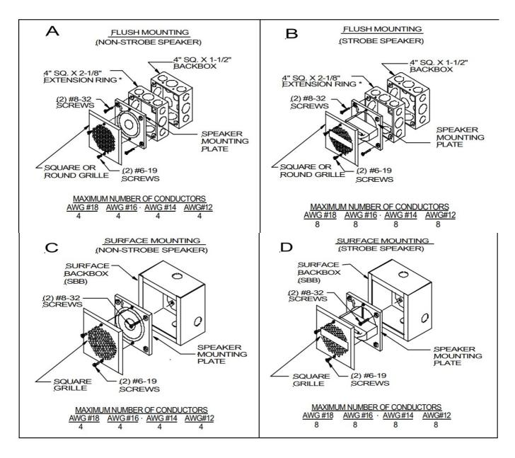
**NOTE:** Surface backbox (SBB) in Figures C & D, is compatible with wiremold and conduit, mounting holes are for single-gang, doublegang, 4"sq., 3-1/2" & 4" octagon or round backboxes.
