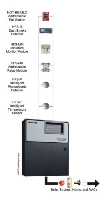
HFS-T: Honeywell Fire Systems addressable fixed temperature heat detector. Includes base.
