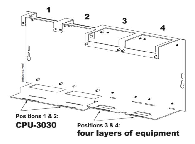
It is critical that all mounting holes of the NFS-3030 are secured with a screw or standoff to ensure continuity of Earth Ground.
