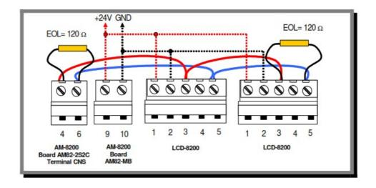
Typical RS.485 connections with 24Vdc common (24V power supply voltage of the control unit)
