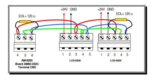
Typical RS485 connections with independent 24Vdc power (LCD panels are powered by remote auxiliary power supplies).
