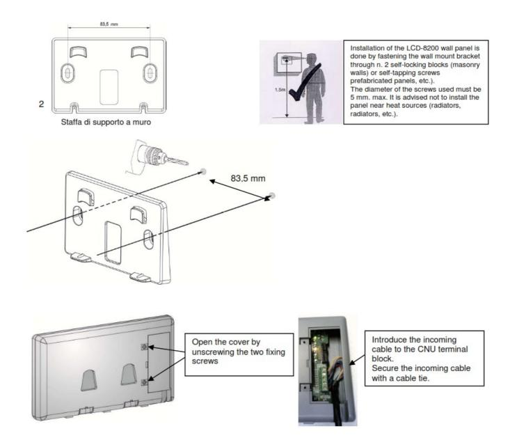
It is recommended not to install LCD-8200 panels near heat sources (radiators, radiators, etc.).
