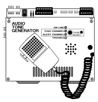
The ATG-2 provides user-selected tones for single- or dual-channel output. The ATG-2 generates either a slow whoop, Hi/Lo or steady tone on the primary (EVAC) channel. In dual-channel operation, the ATG-2 also generates either a chime or a 20 pulses-per-minute tone on the secondary (ALERT) channel.
