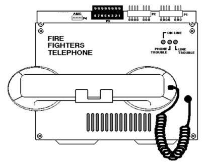
**On Line:** This green LED illuminates to show that the AM2020 is powering the Fire Fighters Telephone system. **Phone Trouble:** This yellow LED illuminates to indicate a trouble in the Fire Fighters Master Telephone (FFT-7S) Circuit.
