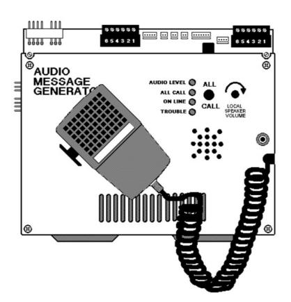
**Audio Level:** This green LED is illuminated when the audio level is correct. When paging, talk loudly enough to cause this LED to illuminate. If the AUDIO LEVEL LED is allowed to remain off for 30 seconds a system trouble will result.
