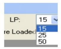
To adjust the Low Pass filter, click on the drop-down box labeled LP. This filter will allow you to reduce muscle noise and electrical artifact.
