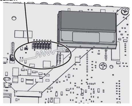
THE ANTENNA SHOULD BE AT THIS ANGLE AFTER TRANSCEIVER INSTALLATION
