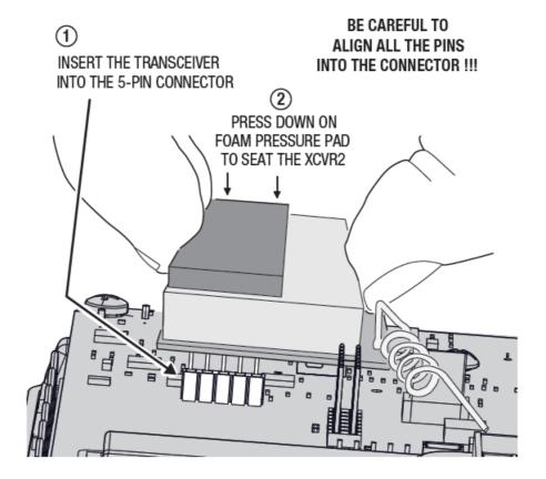
BE CAREFUL TO ALIGN ALL THE PINS INTO THE CONNECTOR !!!
