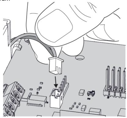
RE-CONNECT THE BATTERY, CLOSE THE CONTROL PANEL, THEN PLUG IN THE AC POWER SUPPLY
