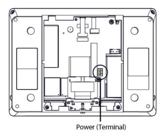
**IMPORTANT:** Never connect the plug-in power supply to a switch-controlled outlet. Do not over-tighten the terminal block's contact screws.
