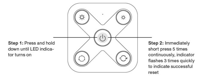
5. Remove a Touchlink paired Zigbee lighting device
