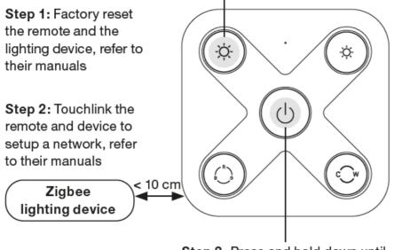
Step 3: Press and hold down until LED indicator turns on
