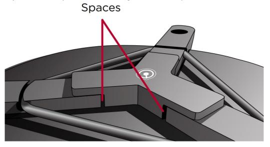
Flip the unit over and set on three Sort Kones so the tips fit into the depressions.
