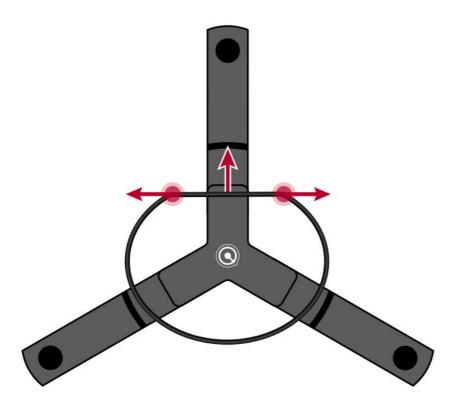
With the grooves facing up, take the rubber ring and stretch it with both hands so that it can snap into the groove on one of the legs.
