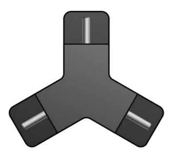
Slide 3 legs onto pins with the slot for the rubber gasket and the Sort Kone depressions facing down
