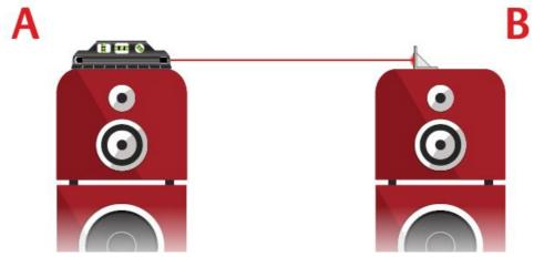
5. USE THE ADJUSTMENT TOOL TO TURN FINIAL DOMES UNTIL THE LASER BEAM MATCHES UP WITH CROSSHAIRS ON TARGET ON SPEAKER 'B'
