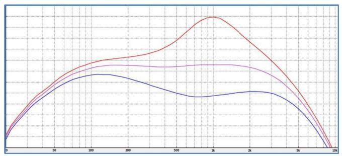
Bonus: When the knob is turned all the way to the right (orange), the clipping (about 3 o'clock position) increases again to counteract the reduced distortion!
