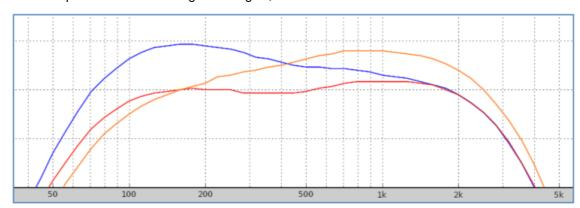
• **Bonus:** If the control is turned all the way to the right (orange), the overdrive (about 3 o'clock position) increases to counteract the reduced distortion!
