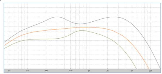
This control 9 has always been special! Unlike other devices on the market (called Tone or Treble), which prune the signal simply in the treble (dull control) I use an active electronics, which regulates not only the treble (from about 1 kHz), but likewise the basses around approx. 300 Hz – so rather the lower middle range.
