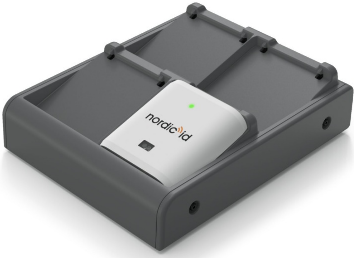
Picture 4 Charging Nordic ID EXA21 via 4-bay desktop charger
