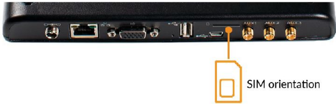
Picture 2 Insertion orientation of mini SIM card
