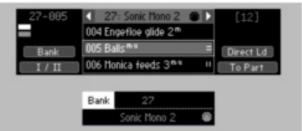
The header of the MIDI-assigned bank is marked by a symbol that looks like a 5-pole MIDI connector. The bank can be connected or disconnected in the following ways:
