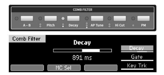
The parameters of the synth engine can be accessed by the 96 selection buttons. The LED of the pressed button will light up. Dots below the LED indicate if additional parameters can be selected by pressing the button multiple times. The stack of selectable parameters is also shown at the right side of the display 19. You can step through it by using the Soft Button as well.
