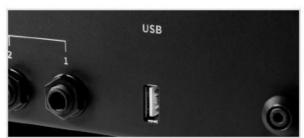
he USB connection is used for plugging in the USB flash drive included with the C15. The drive is used for transferring preset Banks and installing Updates. The C15 comes with its own external power adapter, which connects to the power inlet. A small LED next to the inlet indicates the power, boot and shut-down status of the C15.
