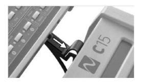
Place the Panel Unit onto the installed Mounting Brackets. The two Mounting Screws on the bottom of the Panel Unit fit into the holes at the top of each Mounting Bracket.
