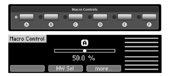
Up to six Macro Controls (MC) can be assigned to modify the sound of a preset. You can access them by their Selection Buttons. Their labels and info can be defined per preset. For the selected MC the LEDs of the target parameters will blink. The MC can be adjusted like a parameter. It can be influenced by Hardware Sources as well, as shown by the eight small bar graphs at the right end of the display 19.
