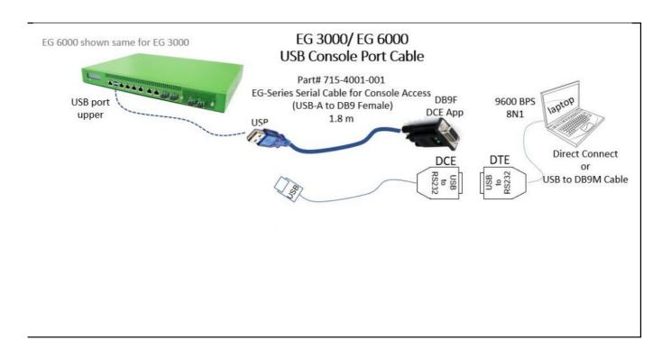
Please note: The EG 6000 Console port only supports asynchronous 9600bps 8N1. Laptop must be configured to match speed.
