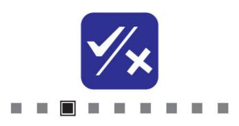
**1-Tone:** In this mode, the device does not discriminate between metals and produces the same sound alert for all metals.
