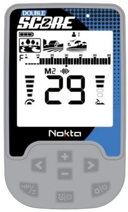
Target ID is shown with two digits on the display and ranges between 01-60. SCORE's Target ID scale consists of 30 lines and each line represents 2 Target IDs.
