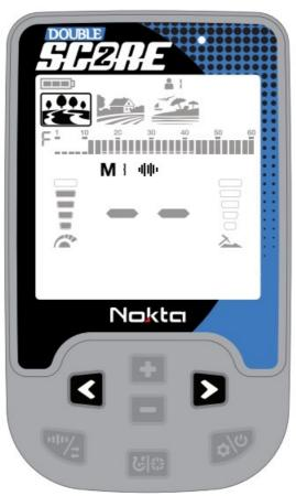
3. You can increase the sensitivity using the Plus (+) & Minus (-) Buttons if needed. Increasing the sensitivity will offer you greater depth. However, if the surroundings or the ground cause excessive noise in the device, you need to lower the sensitivity setting.
