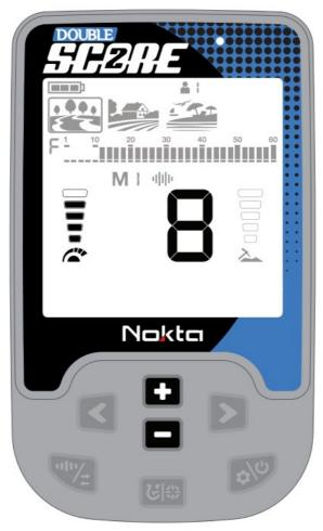
The Sensitivity Indicator is located on the left side of the Target ID. The indicator consists of 5 bars. Each bar represents 2 levels of sensitivity for DOUBLE SCORE and 1 level of sensitivity for SCORE. The sensitivity values corresponding to each level on the Sensitivity Indicator are shown below:
