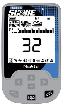
The device updates the ground balance automatically as long as the search coil is swung over the ground. It does not provide any feedback to the user.
