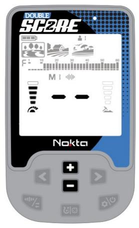
4. If the device receives noise when you increase the sensitivity setting, you can turn on the Noise Cancellation by long pressing the Frequency & Noise Cancellation button before decreasing the sensitivity setting.
