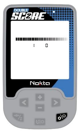
2. When the device is turned on, it will start in the Park mode and in Multi frequency. You can change the mode based on ground conditions. You can find more details on search modes and frequencies further in this manual.
