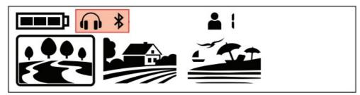
The device will search for the headphones it has been paired with initially and try to connect to those. This will prevent the device from connecting to other Bluetooth® devices when the Bluetooth® setting is on. If you want to pair the device with different Bluetooth® headphones (other than those it was initially paired with) you must delete them from memory.
