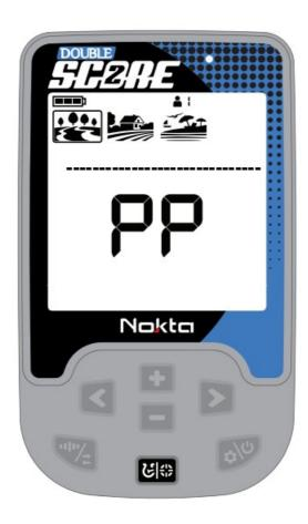
In the pinpoint mode, the device does not discriminate metals or provide Target IDs.
