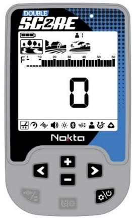
You can navigate through the settings using the Right & Left Buttons. You can adjust the value of a setting using the Plus (+) & Minus (-) Buttons. Press the Power & Settings Button once to exit the settings menu.
