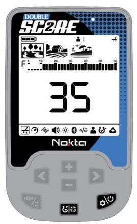
6. If you cannot ground balance, it means that either the ground is too conductive or not mineralized or there is a target right below the search coil. In such a case, retry ground balancing at a different spot.
