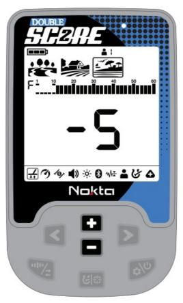
The zero (0) level of the Ground Balance represents the most stable level. Decreasing the Stability level towards -5 may increase the noises originating from beach sand and enhance the probability of detecting weak conductive metals like gold, which give an 11 ID.
