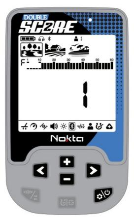
When the wireless connection is turned on, the Bluetooth Headphones icon will start blinking in the info section at the top of the screen.
