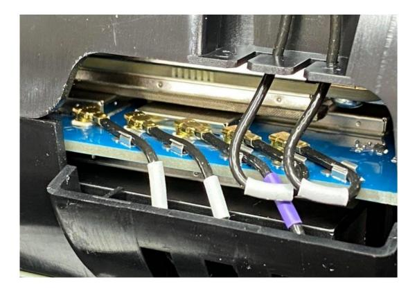
Step 10: Install your U.FL-male to N-female pigtail adapters, in the ports you opened up in step 9.
