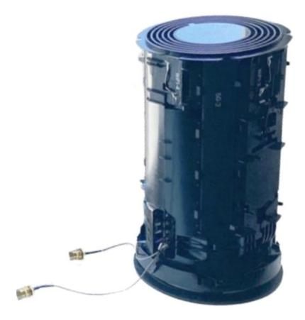
Your T-Mobile 5G Internet Gateway should now be fully re-assembled, with the pigtail adapters protruding from the bottom.
