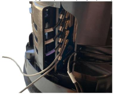
**Step 11 (optional):** Use electrical tape to secure your pigtail adapters to the frame. **Step 12:** Reassemble everything in reverse order. Make sure that your power button is in the off position before reconnecting the battery.
