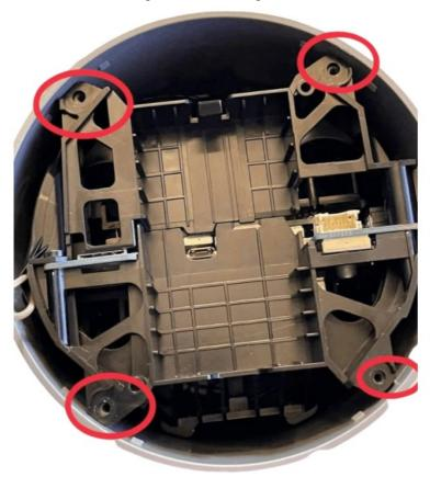
**Step 6:** Work your plastic prying too around the inside edge of the case where it meets the bottom stand, to release the tabs.
