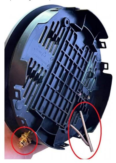
**Step 9:** Rotating the gateway you will see a series of cables connected to the board coming from the antennas. Disconnect the two cables to the right of the purple one, using your prying tool or a pair of tweezers. **Note:** There are a total of four U.FL connectors on the board, two on either side of the purple GPS connector. If you have two MIMO Antenna Kits, you can connect all four U.FL ports for an external 4×4 MIMO setup.
