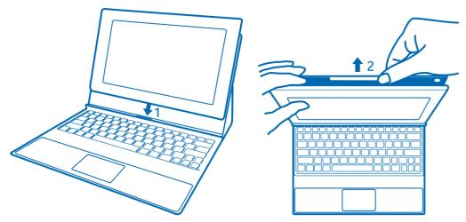
Your tablet uses the cover battery, and switches to use the tablet battery only after the cover battery is empty. Do not fold your tablet holder under the keyboard, as it may damage the cover.
