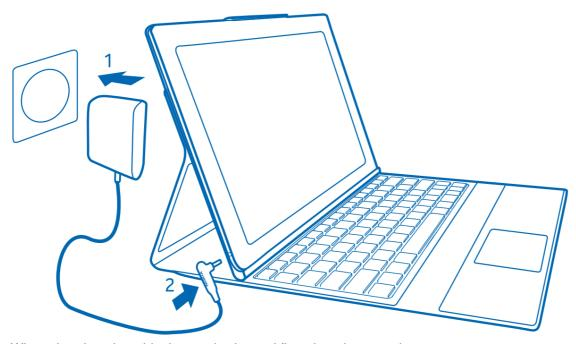
When charging, the tablet battery is charged first, then the cover battery.
