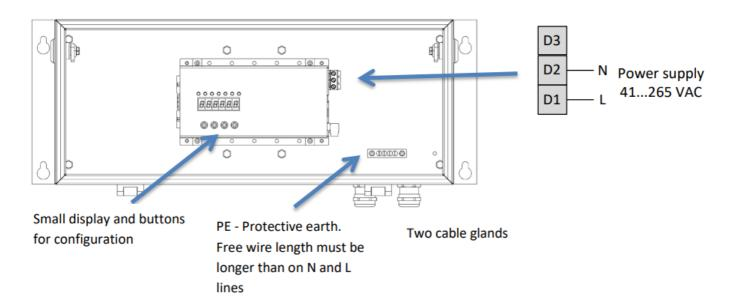
Do not strip the wires more than necessary in order to avoid exposing dangerous voltages. Tie the N and L wires so that if one of them gets accidentally disconnected, the wire end can't reach the other connectors.
