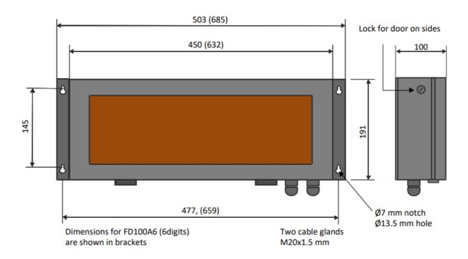
The display unit can be mounted with four screws, one at each corner. The diameter of the screw must be between 5.5 and 6.5 mm. The unit may be mounted to a steel or aluminum structure, to wood with minimum thickness of 20 mm, or to a material of equivalent or better strength.
