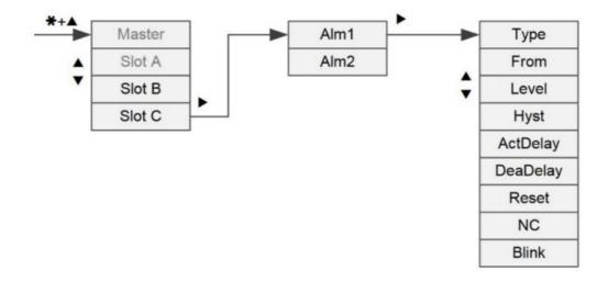
There are two identical submenus, corresponding to two relays.
