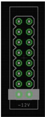
To power your Noise Engineering module, turn off your case. Plug one end of your ribbon cable into your power board so that the red stripe on the ribbon cable is aligned to the side that says -12v and each pin on the power header is plugged into the connector on the ribbon. Make sure no pins are overhanging the connector! If they are, unplug it and realign.
