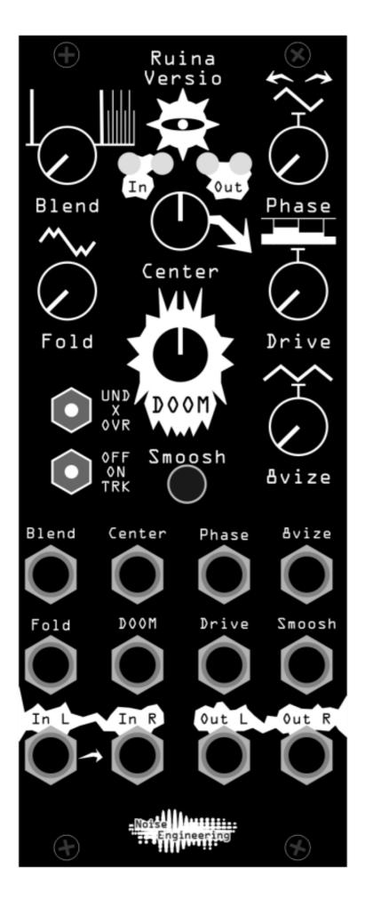
**Blend:** Dry/wet balance control. When turned fully left, the unmodified input signal is passed through. Fully right, only the processed signal is heard. Points in the middle give you a mix of both.
