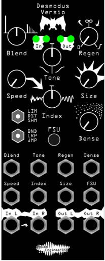
All CV inputs expect 0-5 V. All pots act as offsets and sum with the input CV. The FSU gate input responds to signals above +2 V. The audio inputs clip around 16 V peak to peak.
