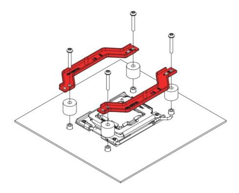
On AM5 and Ryzen 5000/3000 series AM4 CPUs, choose the -7mm offset hole position to ensure optimal contact quality and performance.
