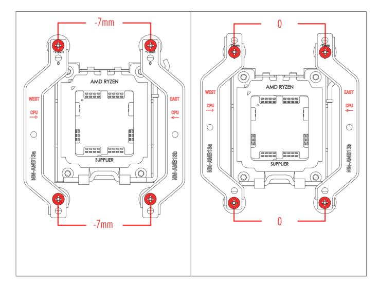
**Caution:** Make sure that the "CPU  $\rightarrow$ " markings point towards the CPU and that the NM-AMB13a bar with the "WEST" marking is installed on the west (left) side of the socket and the NM-AMB13b bar with the "EAST" marking is installed on the east (right) side of the socket.
