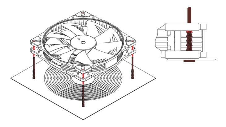
• If the long ends of the mounts are in the way, you can use scissors to cut them after installation. Note that this will then make them difficult to reinstall in the future.
