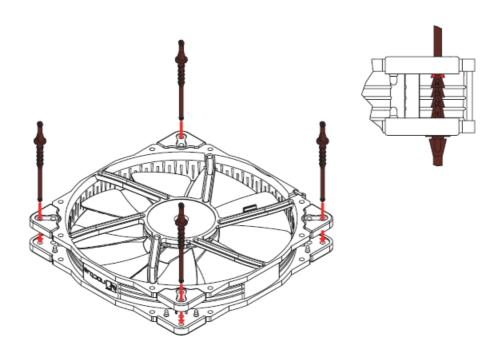
• Then pull the C side through the mounting holes of the case.
