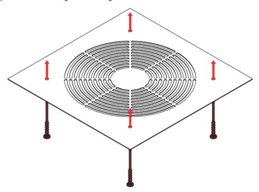
2. Then pull the tip through the fan's mounting holes until the pawl 1 is through the hole.
