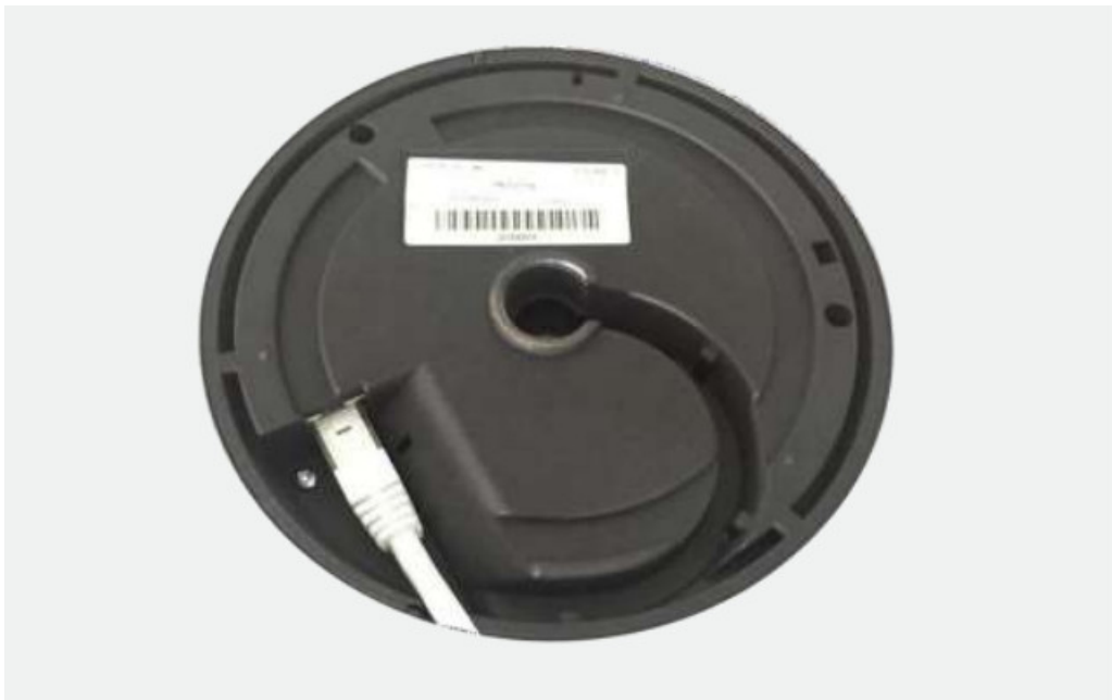
figure 2: Beacon with CAT6 Cable PoE Port
