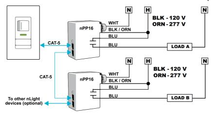
• WIRING to n LIGHT ENABLED DIGITAL LUMINAIRE (e.g. RTLED)
