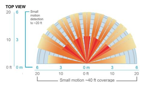
• Coverage pattern shown is derived from NEMA WD7 testing
