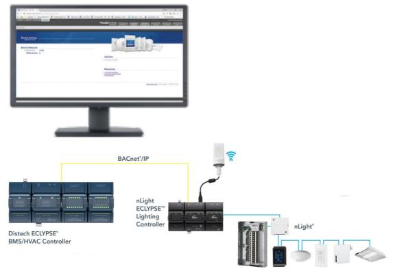
Lightnetwork connects to nECY via onboard light port alight AIR network connects to NECY wa NECYD NLTAIR G2 adapter connected to ECY USB port).
