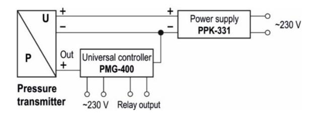
Wiring of 2-wire Ex ia pressure transmitters
