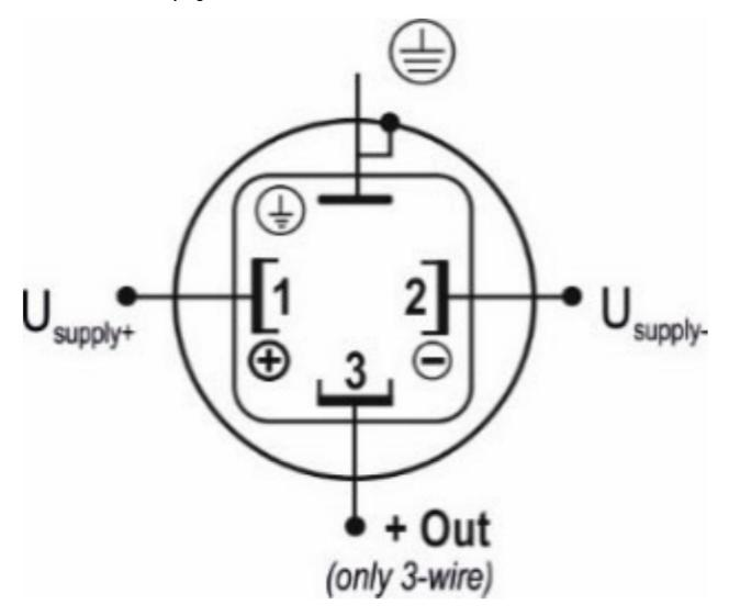
• Connection of M12x1 / 4 pin plug
