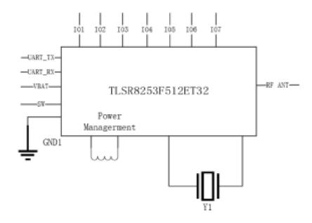
It embeds Flash, LDO and DCDC, crystal, RF match network and etc. With the high integration level of the module, few external components are needed to satisfy customers' ultra-low cost requirements.
