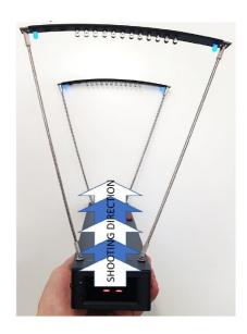
5. Keep end of the rifle barrel around 80cm (or more) distance from the Chronograph. It will prevent non-burned powder pressure wave disturbance for measuring. Avoid direct sun light or sunny days since the UV radiation may disturb the measuring (measuring of Chronograph is based on the light sensors). NOTE: Usage of suppressor, silencer may affect speed readings even with same loading. Do not shoot the Chronograph!
