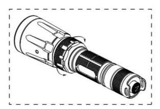
With the light turned on, slowly rotate the Smart Selector Ring (adjacent to the bezel) in a counter-clockwise direction to cycle through the following brightness levels: Beacon -> Police warning signal -> Blue mode -> Green
