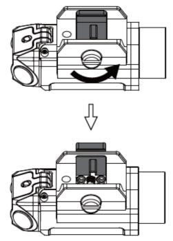
2. Align the stopper with the recoil groove of the rail.
