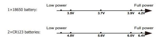
**Note**: when using two CR123/RCR123 in series, the flashlight only reports the average voltage between the two batteries.
