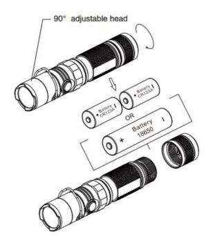
The head of MT21C can be adjusted from 0°- 90° based on users' need.
