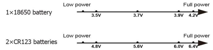
**Note:** When using two CR123/RCR123 in series, the indicator will show the average voltage between the two batteries.
