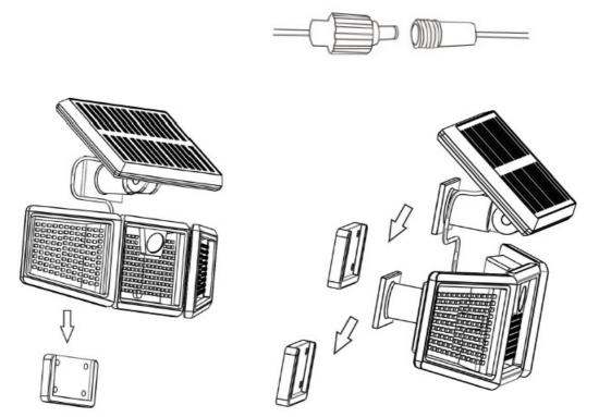
• (**Note:** The connecter needs to be accurately installed in place to achieve the best charging effect and waterproof effect.)
