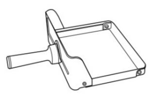
**ASSEMBLY INSTRUCTIONS:** Permanently attach the handle to the baking tray by screwing it clockwise until fully attached.
