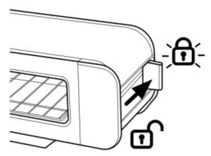
3. **Mode Indicator lights:** Signify Oven or Toaster orientation. Flip the unit down and slide the lever back until it clicks into place to lock the toaster in oven position.
