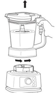
7. Remove the pitcher from the motor base by turning it counterclockwise and then lifting up.
