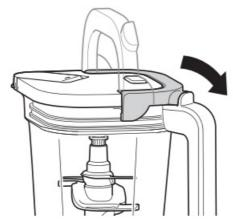
5. Place the lid on the pitcher. Press down on the handle until it clicks into place. Once the lid is locked in place, press the Power button to turn unit on. The available program buttons will illuminate and the unit will be ready for use.
