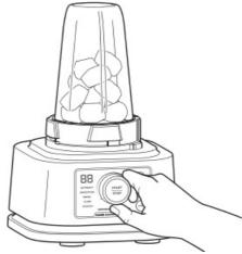
5. a If using an Auto-iQ program, use the dial to select the program that best suits your desired output, then press START/STOP. The preset feature will automatically stop at the end of the program. To stop the unit at any time, press START/STOP.
