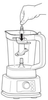
3. Exercising care, grasp the Dough Blade Assembly by the top of the shaft and place it onto the drive gear inside the pitcher. Note that the blade assembly will fit loosely onto the drive gear.
