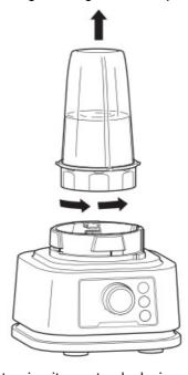
6. Remove the cup from the motor base by turning it counterclockwise and then lifting up.
