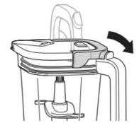
5. Place the lid on the pitcher. Press down on the handle until it clicks into place. Once the lid is locked in place, press the Power button to turn unit on. The available program buttons will illuminate and the unit will be ready for use.
