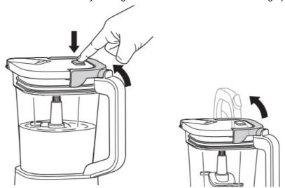
8. Remove the lid and Dough Blade Assembly before removing contents. To remove the lid, press the RELEASE button and lift the handle. To remove the blade assembly, carefully grasp it by the top of the shaft and pull straight up. The pitcher can then be emptied.
