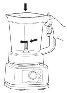
2. Lower the Pitcher onto the motor base. The handle should be aligned slightly to the right and the pitcher should be oriented so the LOCK symbols are visible on the motor base. Rotate the pitcher clockwise until it clicks into place.
