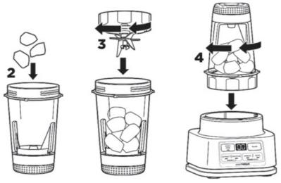
4. Turn the bowl upside down and install on the motor base by aligning the tabs on the bowl with the slots on the base. Then, rotate bowl clockwise until it clicks. Once locked in place, the programs will illuminate and the unit will be ready for use.
