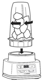
4. Turn the cup upside down and install on the motor base by aligning the tabs on the cup with the slots on the base. Then, rotate cup clockwise until it clicks. Once locked in place, the programs will illuminate and the unit will be ready for use.
