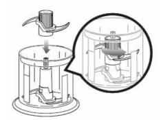
4. Carefully insert the Upper Chopping Blade Assembly over the Lower Chopping Blade Assembly rotating it until it locks onto the Lower Chopping Blade Assembly.
