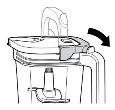
5 Place the lid on the pitcher. Press down on the handle until it clicks into place. Once the lid is locked in place, press the Power
