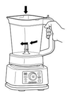
2 Lower the Power Pitcher onto the motor base. The handle should be aligned slightly to the right and the pitcher should be oriented so the LOCK symbols are visible on the motor base. Rotate the pitcher clockwise until it clicks into place.
