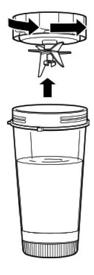
3 Place the Hybrid Edge  $^{\text{TM}}$  Blades Assembly on the top of the bowl and turn clockwise to seal.
