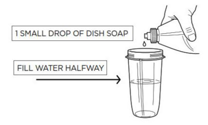
Fill with warm water up to the top of the Power Paddle and add 1 or 2 small drops of dish soap. Install blade assembly.
