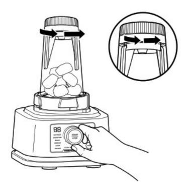
NOTE: While processing, twist the paddle counterclockwise continuously.
