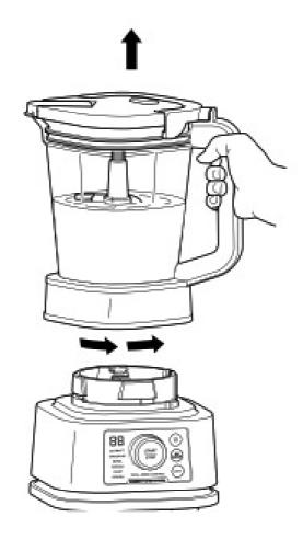
6 Remove the cup from the motor base by turning it counterclockwise and then lifting up.
