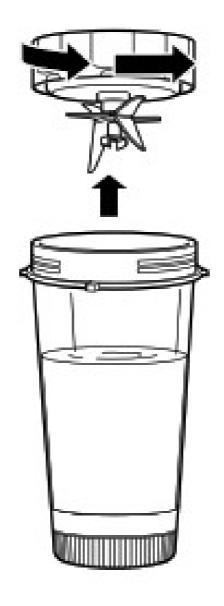
7 Remove the blade assembly by twisting counterclockwise. DO NOT store blended contents with the blade assembly attached. Only use the Spout Lid or Storage Lid to cover. Exercise care when handling the blade assembly, as the blades are sharp.
