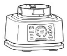
6 Remove the bowl from the motor base by turning it counterclockwise and then lifting up.
