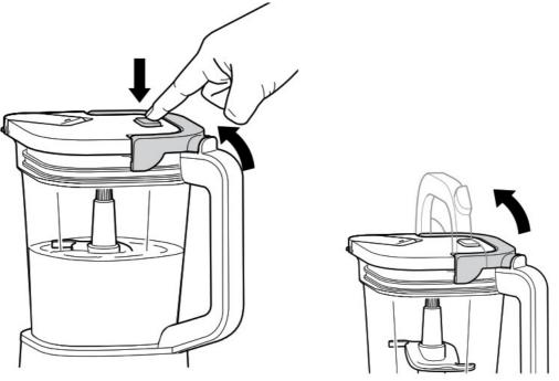
8 Remove the lid and Dough Blade Assembly before removing contents. To remove the lid, press the RELEASE button and lift the handle. To remove the blade assembly, carefully grasp it by the top of the shaft and pull it straight up. The pitcher can then be emptied.
