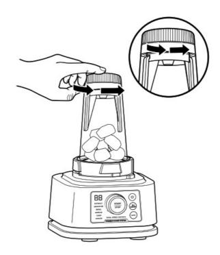
Powering through tough and frozen ingredients used to require a lot of stopping, scraping, and recipe tinkering. But now, it's easier than ever to create thick and spoonable smoothie bowls, nut butter, and more. All you have to do is twist the Power Paddle while blending to push ingredients down toward the blade. It's like having a built-in tamper.
