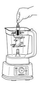
3 Exercising care, grasp the Dough Blade Assembly by the top of the shaft and place it onto the drive gear inside the pitcher. Note that the blade assembly will fit loosely onto the drive gear.
