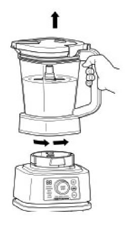
7 Remove the pitcher from the motor base by turning it counterclockwise and then lifting up.
