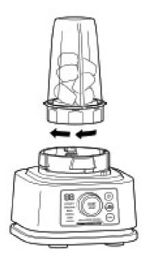
4 Turn the cup upside down and install on the motor base by aligning the tab on the cup with the slots on the base. Then,
