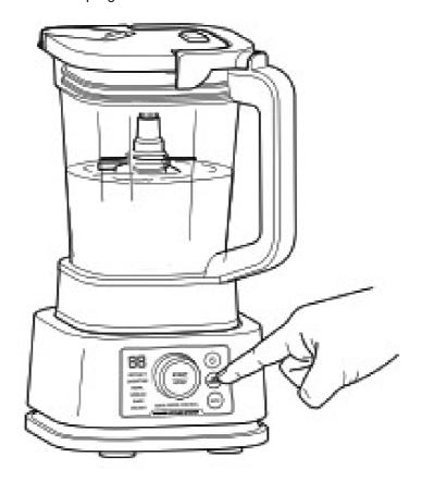
6a If using an Auto-iQ® program, use the dial to select DOUGH, then press START/STOP. The preset feature will automatically stop at the end of the program. To stop the unit at any time, press START/STOP. 6b For Manual mode, press IQ/MANUAL.
