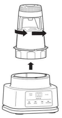
6. Remove the bowl from the motor base by turning it anti-clockwise and then lifting up.
