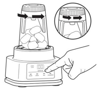
NOTE: While processing, twist the Power Paddle anti-clockwise continuously.
