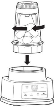
4. Turn the bowl upside down and install on motor base by aligning the tabs on the bowl with the slots on the base. Then, rotate bowl clockwise until it clicks. Once locked in place, press the Power button o turn unit on. The available program buttons will illuminate and the unit will be ready for use.
