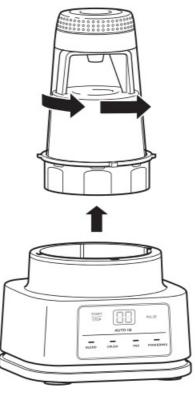
6. Remove the bowl from the motor base by turning it anti-clockwise and then lifting up.
