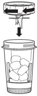
3. Place the Hybrid Edge Blades Assembly on the top of the bowl and turn clockwise to seal.
