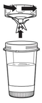
7. Remove the blade assembly by twisting anti-clockwise. DO NOT store blended contents with the blade assembly attached. Only use the Spout Lid or Storage Lid to cover. Exercise care when handling the blade assembly, as the blades are sharp.
