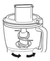
9. Turn the unit off by pressing the Power button. Unplug the unit when finished. Refer to the Care & Maintenance section for cleaning and storage instructions.
