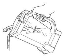
8b For thicker mixtures that cannot be emptied through the pour spout, remove the lid and Total Crushing® Blade before pouring. To remove the lid, press the RELEASE button and lift the handle. To remove the blade assembly, carefully grasp it by the top of the shaft and pull it straight up. The Jug can then be emptied.
