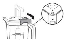
5. Place the lid on the Jug, aligning the triangle symbol on the lid with the triangle symbol on the handle. Press down on the handle until it clicks into place. The triangle symbols MUST be aligned for the lid to lock and the unit to operate. Once the lid is locked in place, press the Power button to turn unit on. The available program buttons will illuminate and the unit will be ready for use.
