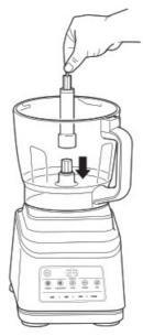
4. Use the finger holes to grasp the disc and place it over the adapter with the side you would like to use facing up.
