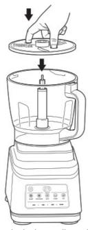
5. Place the feed chute lid on the bowl and turn clockwise until you hear a click, indicating the lid is locked in place.
