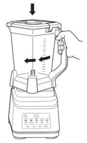
2. Lower the Total Crushing® Jug onto the motor base. The handle should be aligned slightly to the right and the Jug should be oriented so the LOCK symbols are visible on the motor base. Rotate the Jug clockwise until it clicks into place.
