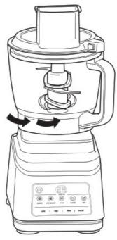
8. Release the lid by twisting anti-clockwise and lifting upwards from the motor base. Ensure the blade is removed before emptying the contents.
