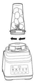
4. Turn the cup upside down and install on the motor base. Align the tabs on the cup with the slots on the base, then rotate cup clockwise until it clicks into place. Once the cup is locked in place, press the Power button to turn unit on. The available program buttons will illuminate and the unit will be ready for use.
